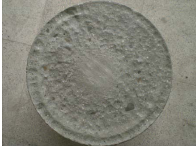
Figure 7 the picture of specimen OPC-S10-0.28-28 after 72 hour abrasion test
