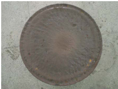
Figure 8 the picture of specimen FOPC-S10-0.28-28 after 72 hour abrasion test
