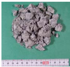
Photo 1 Example of Recycled Crusher-run
