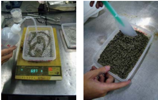
Photo 2 Examination and Adjustment of Moisture Condition[8]
