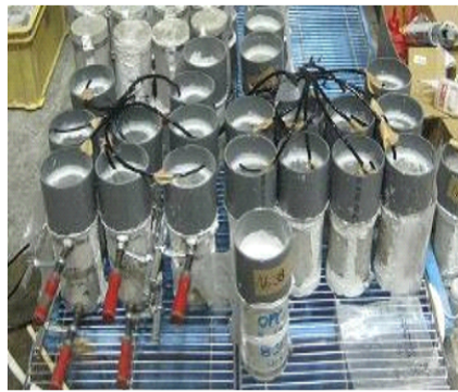
(a) Water permeability test
