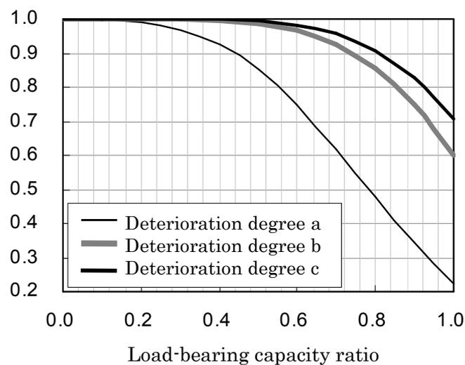
**Fig. 11: Probability of load-bearing capacity ratio exceeding  $x$ <sup>6)</sup>**
