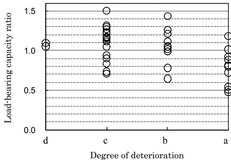
**Fig. 10: Deterioration degree related to load-bearing capacity ratio<sup>6)</sup>**
