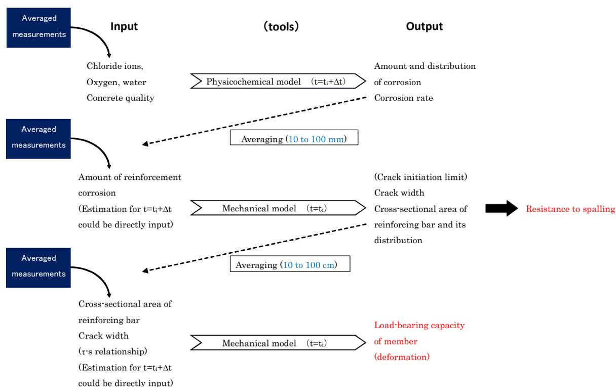
**Fig. 1: Data flow and data averaging from micro- to macro-scale**
