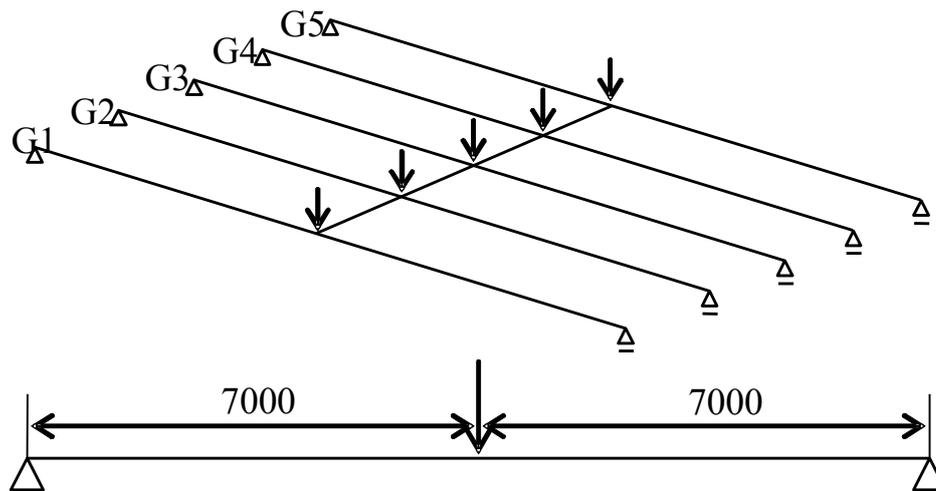
Fig. 9: Arrangement of different corrosion zones in deteriorated girder
