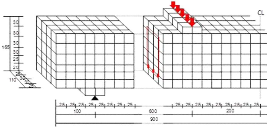
Fig. 6: Analysis model of analyst A
