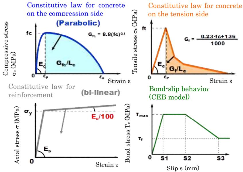
Fig. 5: Constitutive models of materials used by Analysis A
