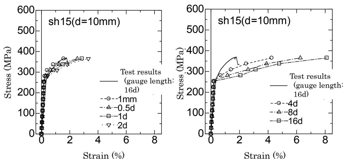
**Fig. 2: Effect of element size on stress-strain relationship**
