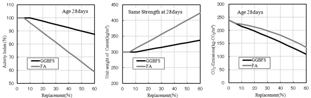
**Fig. 2: Examples of trial calculation of the relations between mortar intensity ratio, unit weight of cement and CO<sub>2</sub> emissions in relation to a replacement rate with blast-furnace slag or fly ash**
