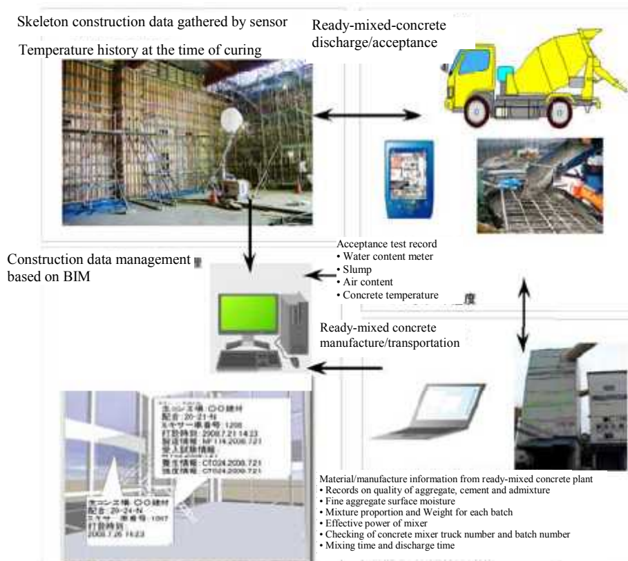
Fig. 8: Construction data collection and integrated image by use of BIM
