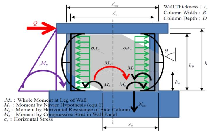
**Fig. 3: Assumed bending moment produced in wall legs**
