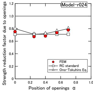
**Fig. 9: Comparison example of strength reduction ratio due to openings (horizontal axis values are the distances from the wall centers to opening centers divided by  $\frac{1}{2}$  of the entire wall)**
