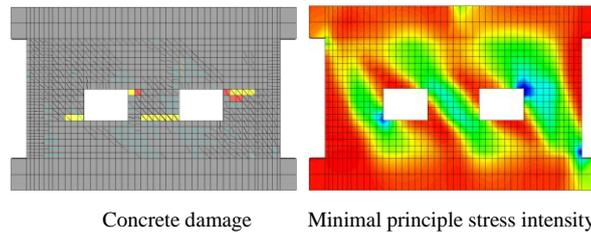
**Fig. 8: Example of analysis of perforated wall member receiving horizontal force**
