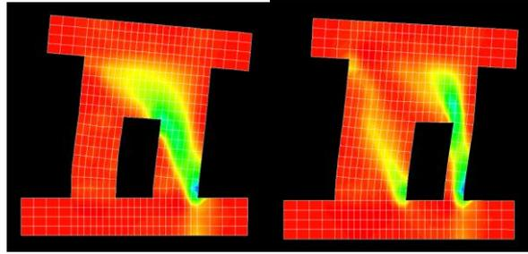
**Fig. 7: Minimal principle stress intensity contour during maximum lateral force**
