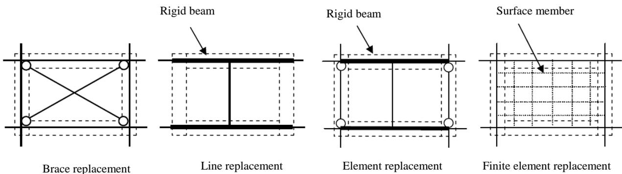
**Fig. 1: Replacement model example of two-column wall**
