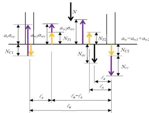
**Fig. 4: Assumed shear force in wall legs**
