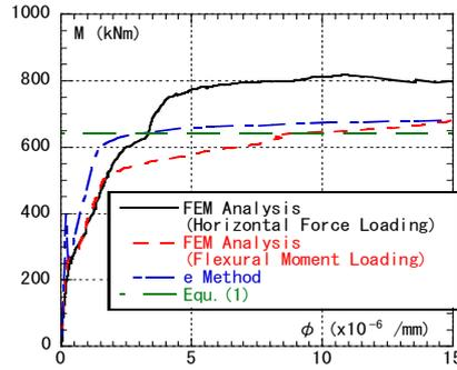
**Fig. 2: Comparison of bending-moment–curvature relationship of wall legs (shear-span ratio 0.99)**
