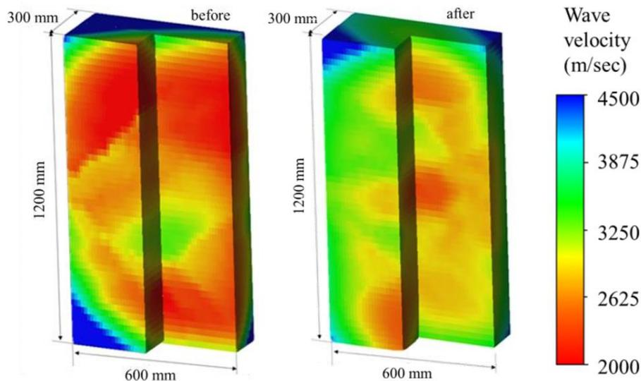
**Fig. 4: Three-dimensional elastic-wave velocity distribution before and after grouting<sup>3)</sup>.**
