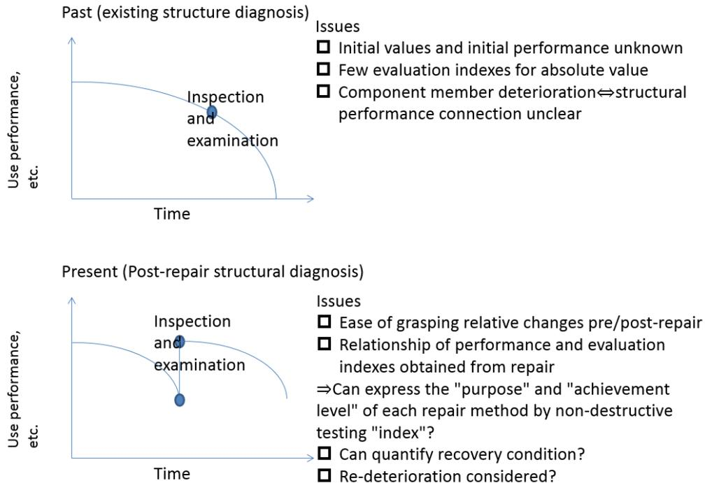
**Fig. 3: Evaluation image of existing structure before and after repair.**
