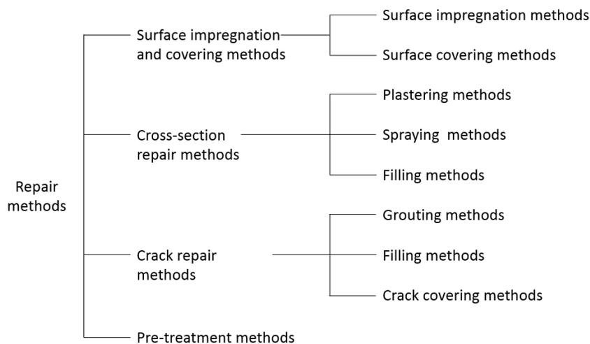
**Fig. 1: Repair methods summarized.**
