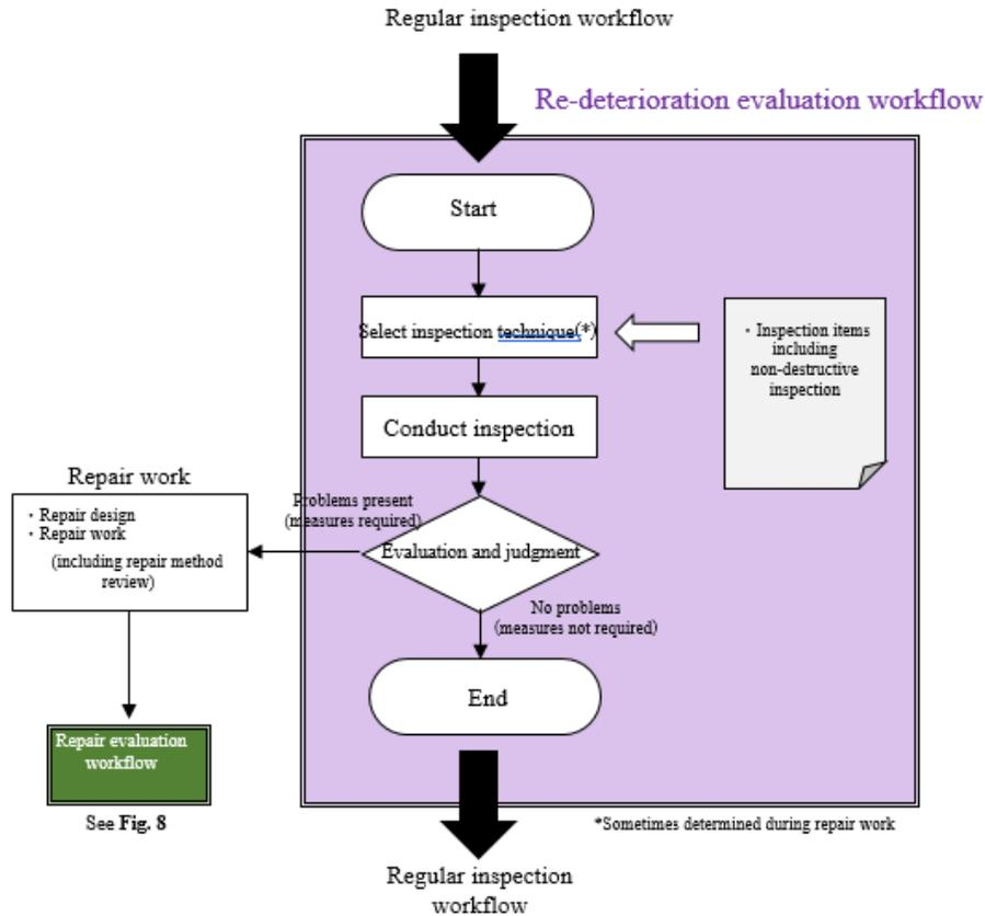
**Fig. 9: Re-deterioration evaluation workflow.**
