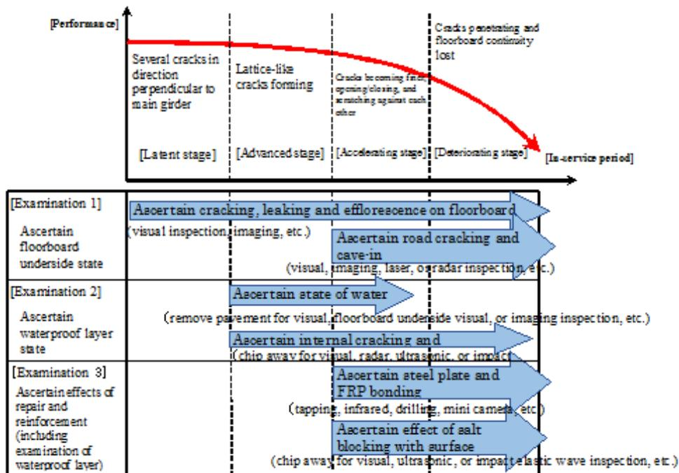
**Fig. 6: Image of deterioration process in the fatigue of slab.**
