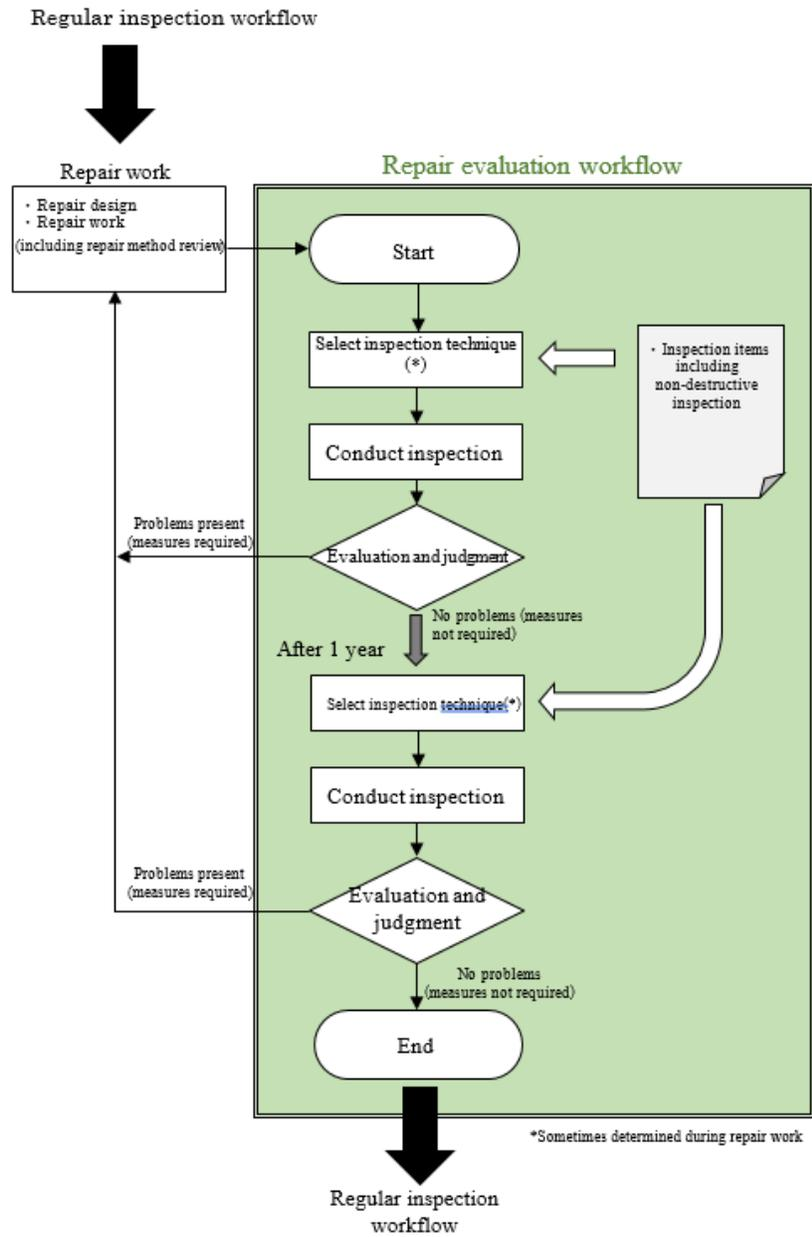
**Fig. 8: Repair evaluation workflow.**
