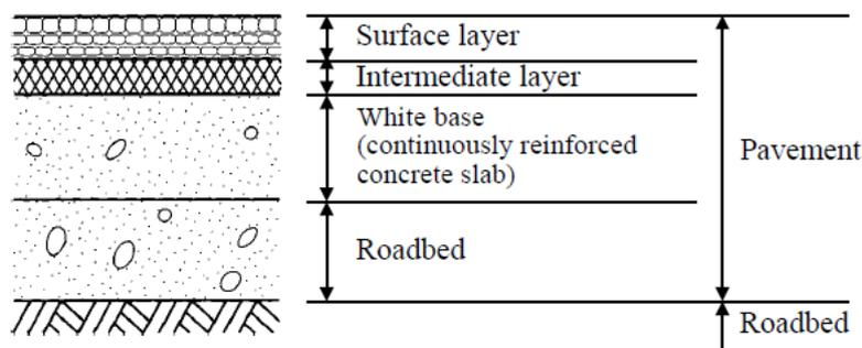
**Fig. 6: Composition of composite pavement in a highway**
