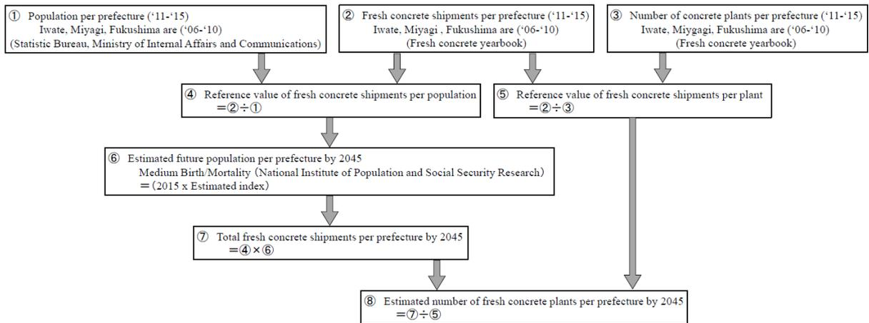
**Fig. 2: Estimation process for future fresh concrete shipments and number of plants (by 2045)**
