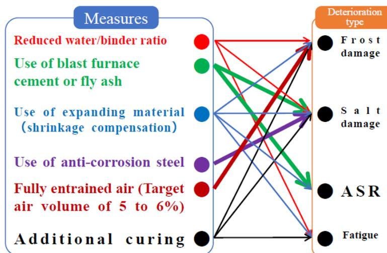
Fig. 5: RC slab durability-increasing measures (Tohoku road reconstruction)
