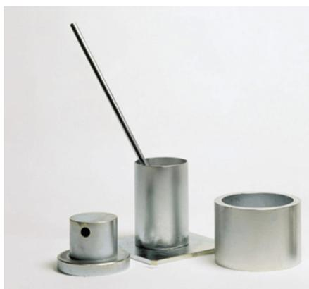
**Fig. 3: Example of BS812-110 test device<sup>2)</sup>**
