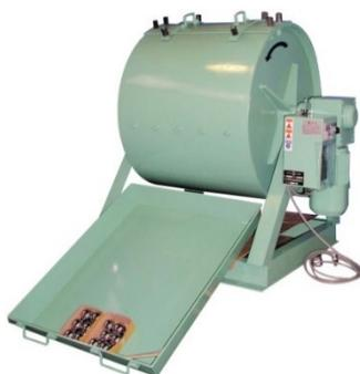
**Fig. 2: Example of Los Angeles test equipment<sup>1)</sup>**
