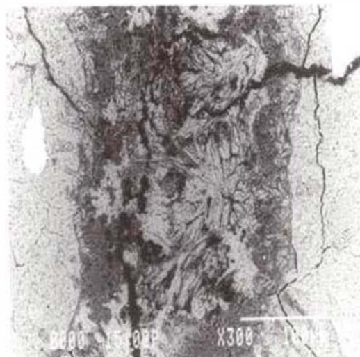
(a) Ettringite and magnesium hydroxide depositing near cracking (courtesy of H. Hamada)
