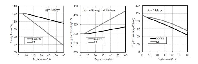
Fig. 2: Examples of trial calculation of the relations between mortar intensity ratio, unit weight of cement and CO<sub>2</sub> emissions in relation to a replacement rate with blast-furnace slag or fly ash
