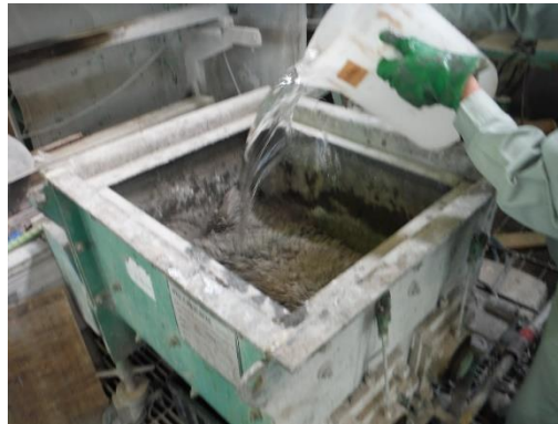
Image 1 - Mixing Geopolymer in a Forced Biaxial Mixer
