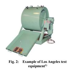
JIS A 1121: "Abrasion test method for coarse aggregate using Los Angeles test equipment" is one of the current standards for aggregate strength and hardness. However, this test method evaluates only the abrasion resistance of aggregate and not its strength.
