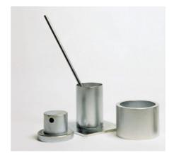
Fig. 3: Example of BS812-110 test device<sup>2)</sup>
