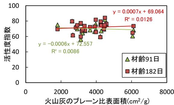
Fig. 3: Blaine’s specific surface area and activity index in JIS A 6201 (W/B = 50%)<sup>5)</sup>
