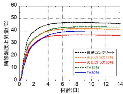
Fig. 10: Adiabatic temperature increase test results
