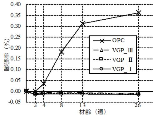
**Fig. 17: Test results by mortar bar method**
