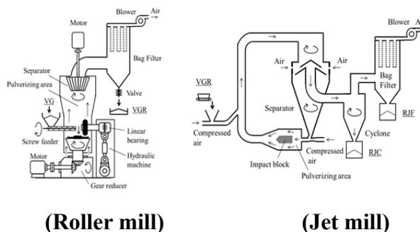
**Fig. 2: Improved roller mill and jet mill<sup>3)</sup>**
