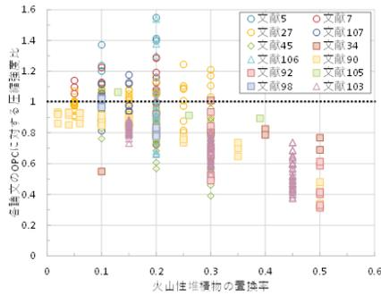
**Fig. 11: Replacement rate of volcanic sediments and compressive strength ratio with respect to OPC (comparison by paper)**
