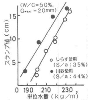
Fig. 7: Relationship between unit water volume and slump
