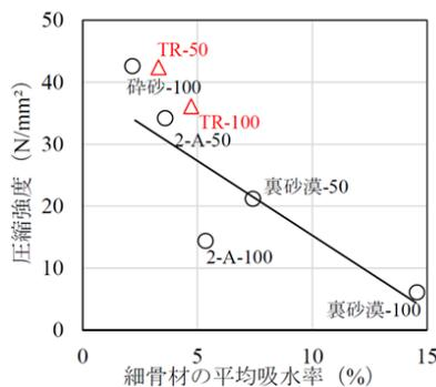
**Fig. 12: Average water absorption and compressive strength of fine aggregate**
