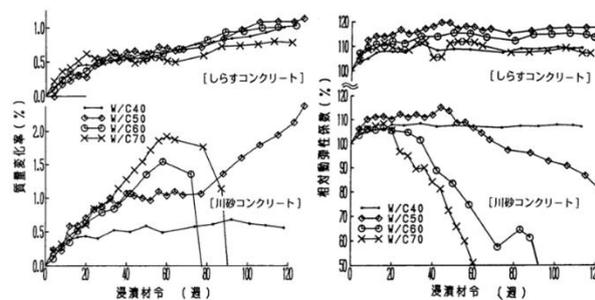
**Fig. 15: Changes in mass and kinematic modulus in 10% Na<sub>2</sub>SO<sub>4</sub> solution**
