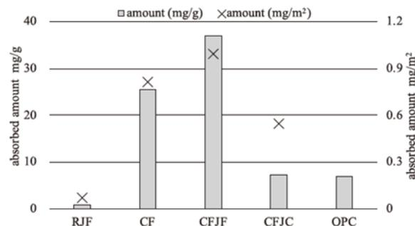
**Fig. 6: Absorption amount of high-performance AE water-reducing agent**
