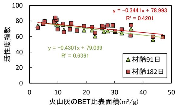
Fig. 4: BET specific surface area and activity index in JIS A 6201 (W/B = 50%)<sup>5)</sup>
