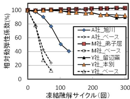
**Fig. 16: Results of water freeze–thaw test**
