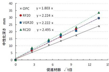
**Fig. 14: Results of accelerated neutralization test of OPC and concrete with an addition replacement rate of 20%**
