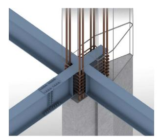
Fig. 5 Beam-to-column connection
