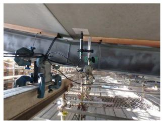
Fig. 13 High-precision displacement transducer
