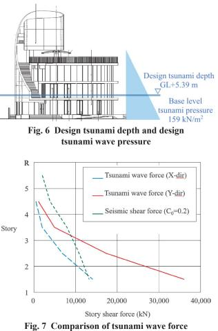
and story seismic shear force
