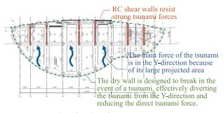
Fig. 10 First-floor beam plan
