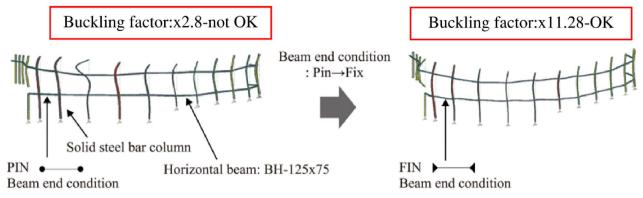
Fig. 6 Results of buckling analysis
