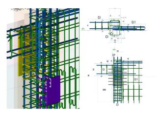
Fig. 9 Step 1: 3D model for rebar
