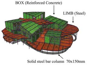
Fig. 4 Structural analysis model
