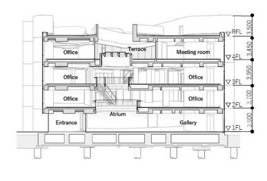
Fig. 2 Architectural plan and section
