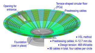
Fig. 2 Structural overview of Cofun A
