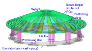
Fig. 3 Structural overview of Cofun C
