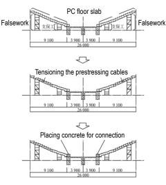
Fig. 9 Construction of Cofun A
