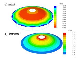
Fig. 6 Cofun C: edge compressive stress (N/mm<sup>2</sup>)
