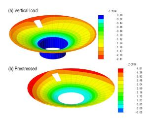
Fig. 5 Cofun A: vertical displacement (mm)
