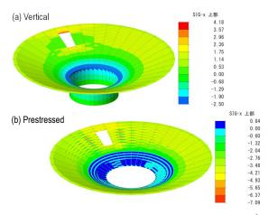
Fig. 4 Cofun A: edge compressive stress (N/mm<sup>2</sup>)
