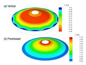
Fig. 7 Cofun C: vertical displacement (mm)
