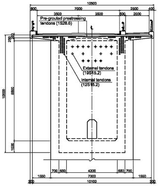
Fig. 2 Cross section at pier head
