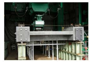
Fig. 3 Wheel load running test
