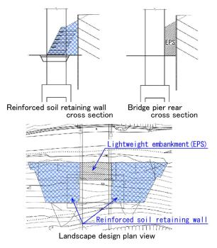
Fig. 3 Use of lightweight embankment
