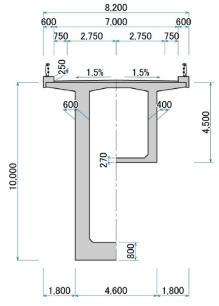
Fig. 5 Cross section of main girder
