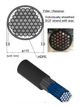
Fig. 3 Stay cable with four-layer corrosion protection
