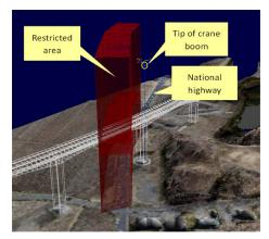
Fig. 7 GNSS crane monitoring system
