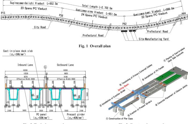
Fig. 2 Typical cross section
