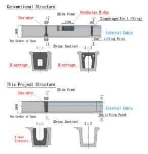
Fig. 7 Comparison of precast girder structures
