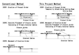
Fig. 9 Comparison of erection methods
