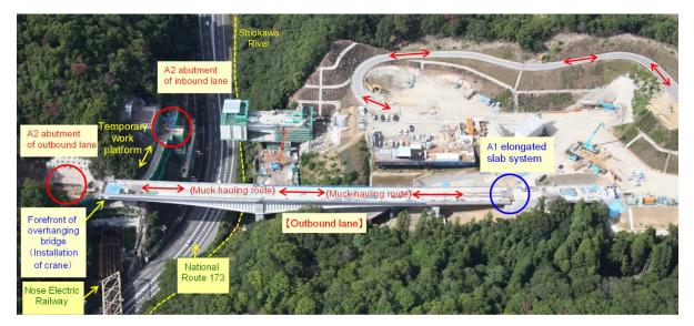
Fig. 7 Transport route of excavated soil at A2 abutment
