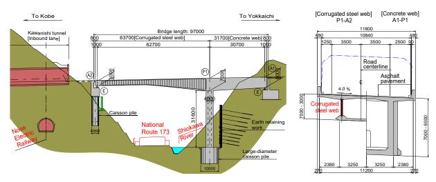
Fig. 2 Overall diagram and standard section of the superstructure of the inbound lane
