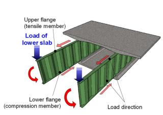
Fig. 5 Load-carrying mechanism lower slab
