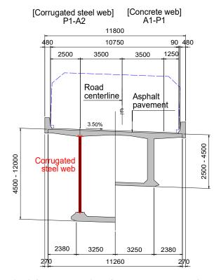
Fig. 4 Standard section of the superstructure of the outbound lane
