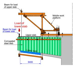
Fig. 6 Load-supporting mechanism of the lower slab concrete
