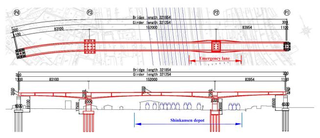
Fig. 3 Overview of Yaga Overpass Bridge
