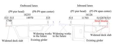
Fig. 3 Main girder cross sections
