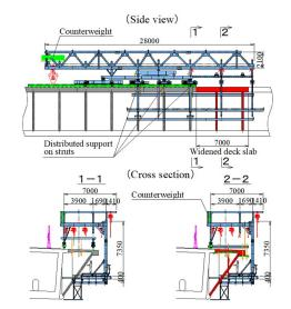
Fig. 10 Mobile overhanging platform
