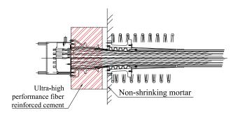
Fig. 6 Anchoring device (UHPFRC)
