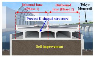
Fig. 2 Conceptual illustration of the renewed section on completion
