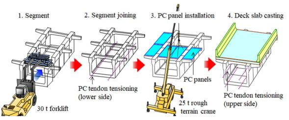
Fig. 4 Box culvert construction processes
