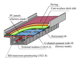
Fig. 3 Overview of the box structure
