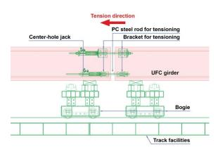
Fig. 5 Joining equipment
