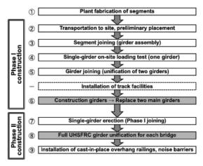
Fig. 3 Construction flow
