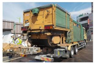
Fig. 9 Jet concrete mixer truck
