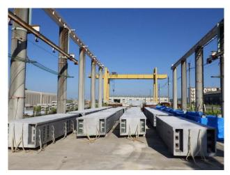
Fig. 4 Fabrication of UFC segments
