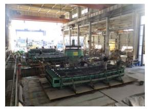
Fig. 8 Manufacturing of precast panels
