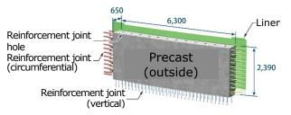
Fig. 5 Image of precast panel (unit: mm)
