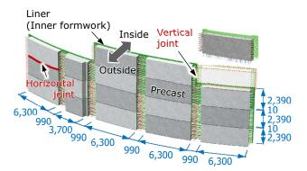
Fig. 6 Joints of precast panels (unit: mm)
