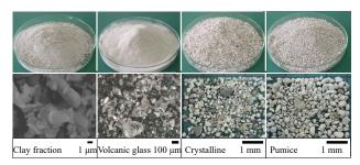
Fig. 2 Four types of mineral after sorting<sup>[1]</sup>
