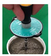
Fig. 2 Vane shear test
