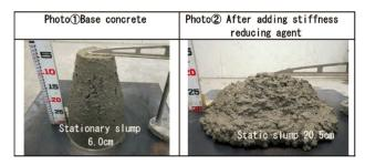
Fig. 1 Comparison of static slump test results
