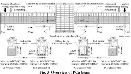
concrete are roughened, and shear keys are formed with inflatable cushions on the cross section of the post-casting concrete in contact with the columns to integrate them with the post-casting concrete.
