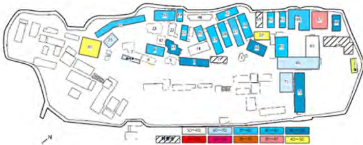
Residual capacity of vertical load
