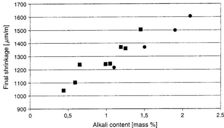
**Figure 7: Final shrinkage of concrete as function of the alkali content (■ Na<sub>2</sub>O and ● K<sub>2</sub>O), (F. Beltzung et al., 2001).**
