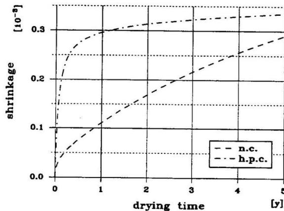
**Figure 10: Evolution of shrinkage of normal (n.c.) and of high performance concrete (h.p.c.) as determined along the axis of the specimens**
