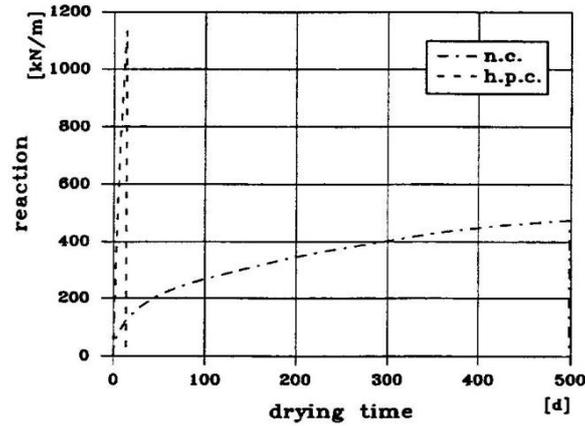
Figure 11: Evolution of restraint reaction of fully restraint members of normal (n.c.) and of high performance concrete (h.p.c.)
