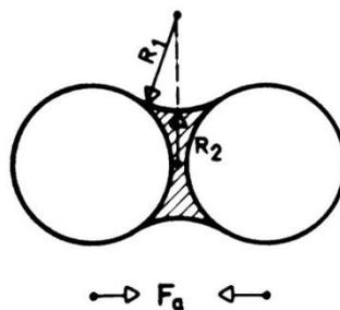
**Figure 3: Water layer between two spherical particles**
