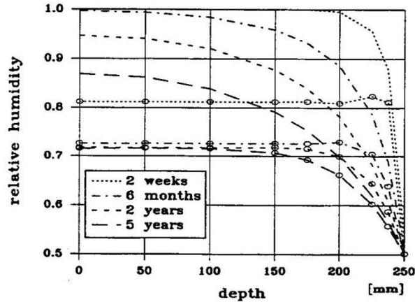
**Figure 9: Moisture distribution in normal and high strength concrete (curves plotted with circles) in the first five years**
