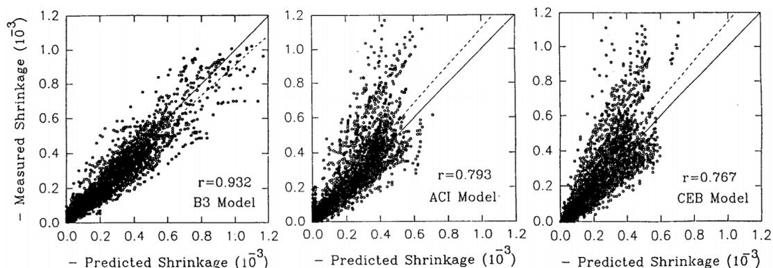
**Figure 1: Scatter plots of measured versus predicted values of shrinkage of concrete, dashed lines are regression lines (Bazant Z. P., and Baweja S., 1995(1)).**
