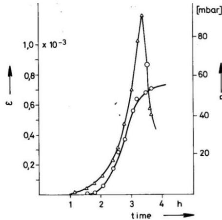
**Figure 2: Evolution of capillary pressure  $p$  in fresh concrete and resulting capillary shrinkage  $\varepsilon$  as function of age of concrete (Wittmann F. H., 1976).**
