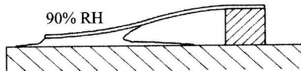
**Figure 4: Thin glass plate separated from the polished quartz support by disjoining pressure of water**
