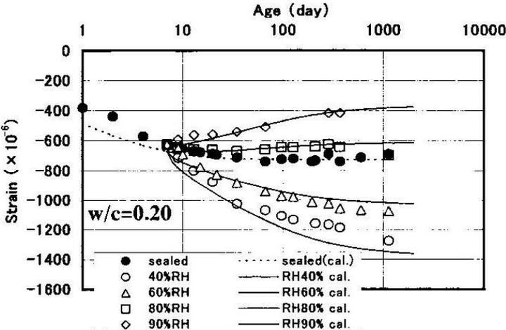
Figure 8: Self-desiccation and autogenous shrinkage of high strength concrete, (S. Miyazawa and E. Tazawa, 2001)
