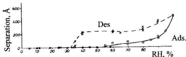
**Figure 5: Distance between the free end of the thin glass plate and the support as function of RH. Both the adsorption and desorption branches are shown.**
