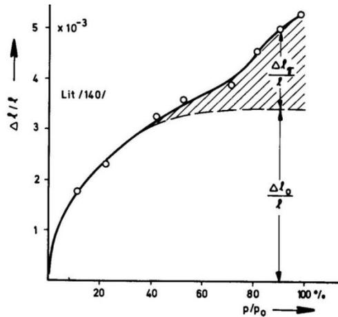
**Figure 6: Hygral length change of hardened cement paste as function of RH.**
