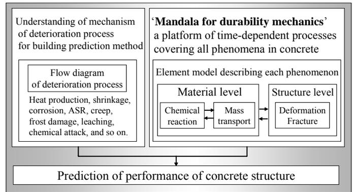
Figure 1. Approach to *durability mechanics*.
