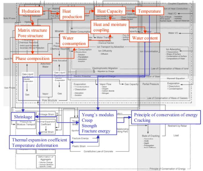
Figure 5. Durability mechanics regarding heat production and shrinkage.
