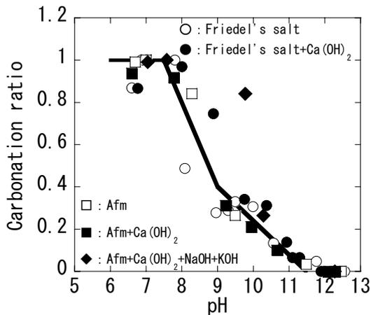
Figure 18. Relationship between pH and carbonation ratio.
