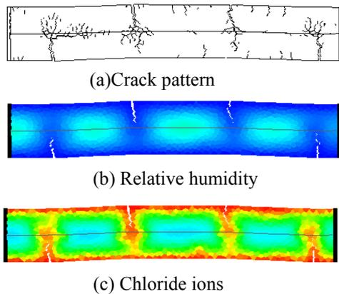
Figure 30. Combined analysis of drying shrinkage and corrosion.
