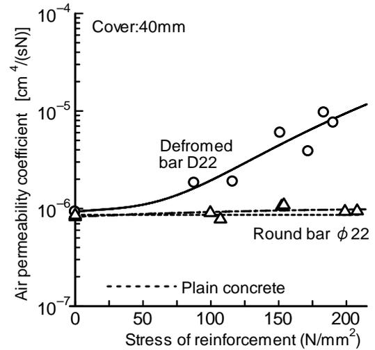
Figure 26. Increase in air permeability coefficient of cover concrete with deformed bar.
