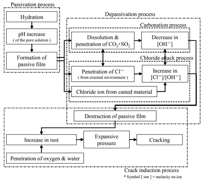
Figure 6. Mechanism of deterioration due to steel corrosion.
