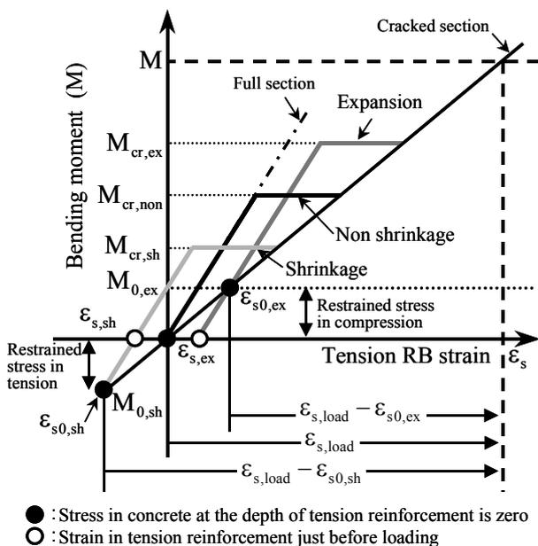
Figure 22. Concept of effect of shrinkage/expansion on strain change in tension reinforcement.
