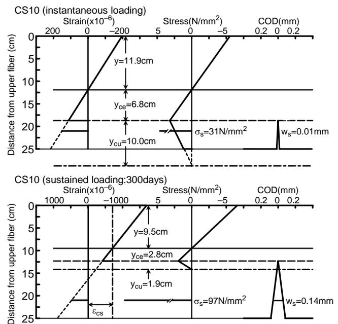
Figure 20. Computed distributions of strain, stress and COD at cracked section.
