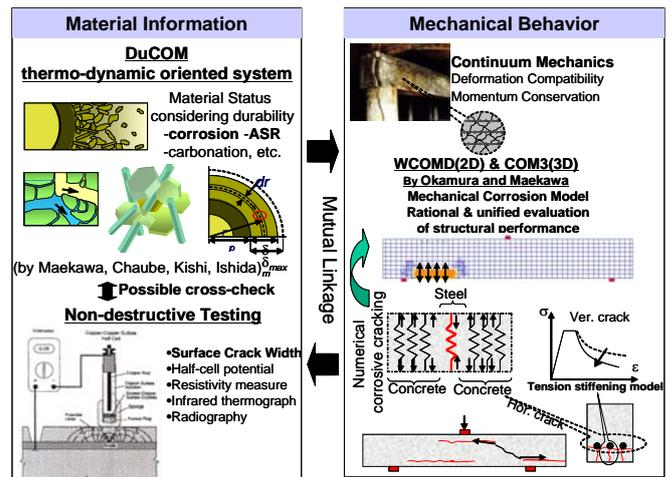
Figure 29. Structural performance assessment of corroded RC.
