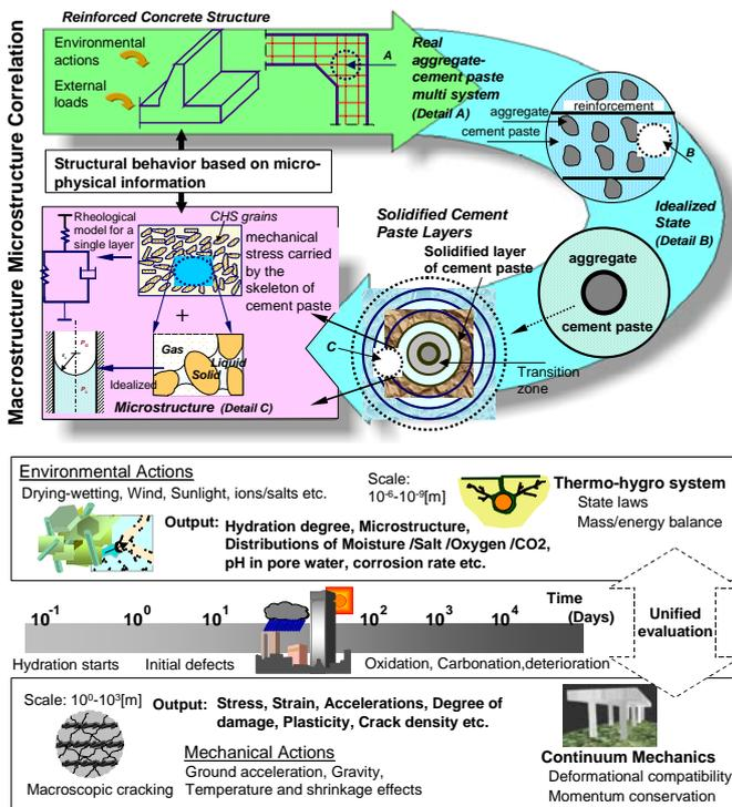
Figure 27. Multi-scale scheme and lifespan simulation for materials and structures.
