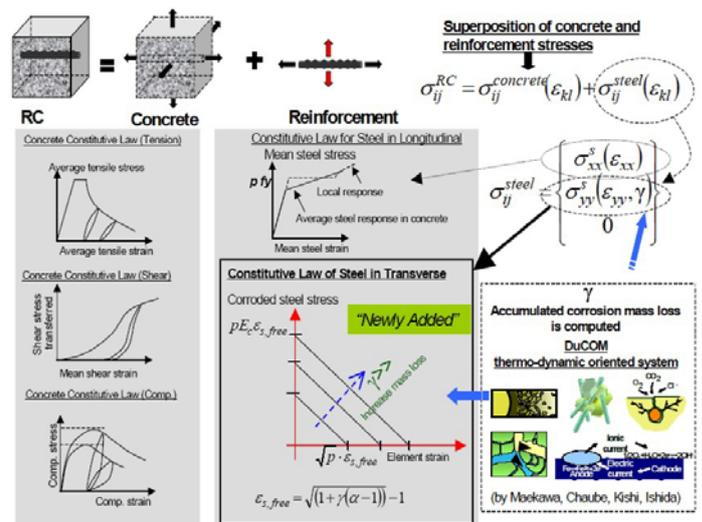
Figure 9. Constitutive models for reinforcement and concrete in RC considering corrosion.
