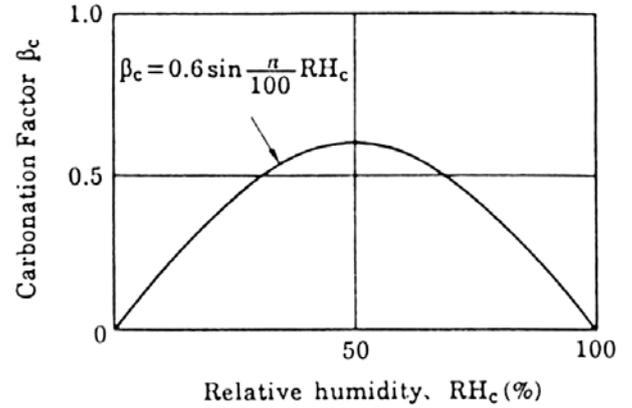
Figure 16. Relation between relative humidity and carbonation factor.
