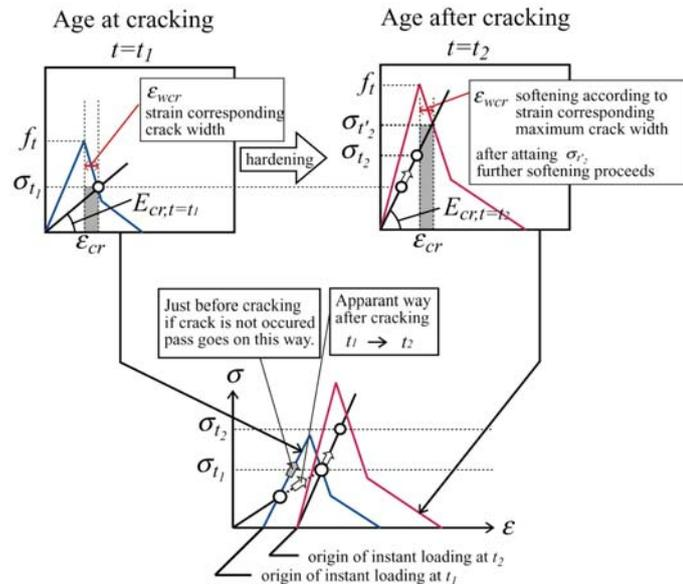
Figure 25. Time-dependent micro-crack model.
