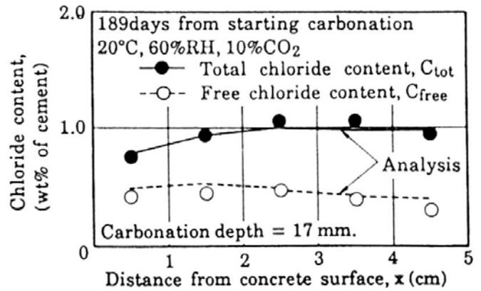
Figure 17. Chloride condensation by carbonation (result of accelerated carbonation test and analysis).
