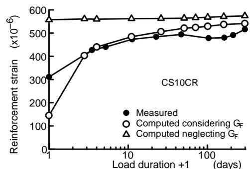
Figure 21. Comparison of measured and computed time-dependent change of maximum strain in tension reinforcement.
