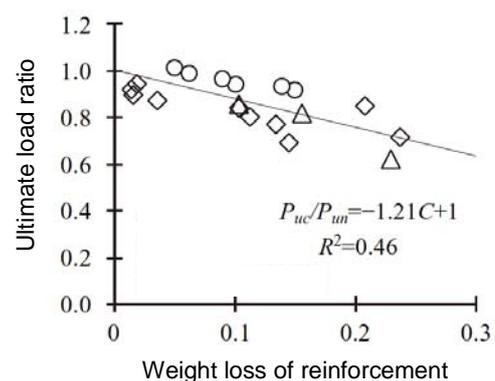
Figure 7. Flexural capacity vs. weight loss in experimental RC members.
