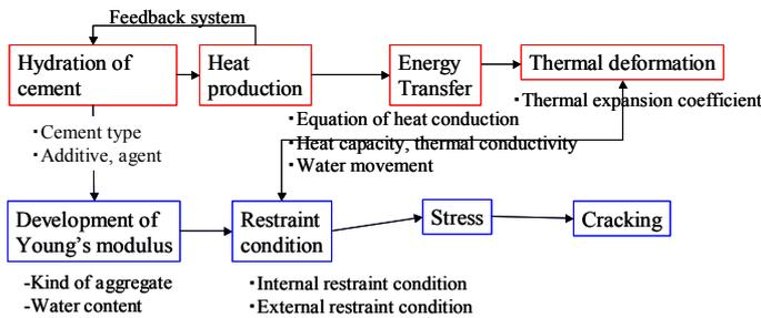
Figure 3. Process of cracking due to heat production.
