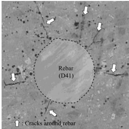
Figure 24. Cracking around reinforcing bar due to autogenous shrinkage.
