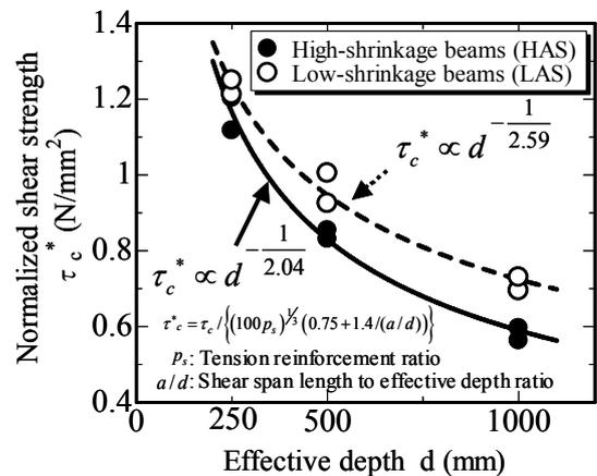
Figure 23. Dependence of size effect on shrinkage for diagonal cracking strength.
