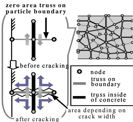
Figure 31. Truss networks.
