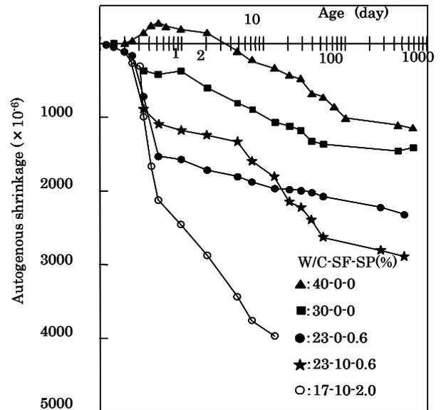
Figure 11. Influence of water-cement ratio on autogenous shrinkage of cement paste.
