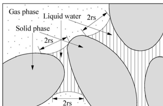
Figure 14. Modeling of pore structure of concrete and behavior of water in pores.
