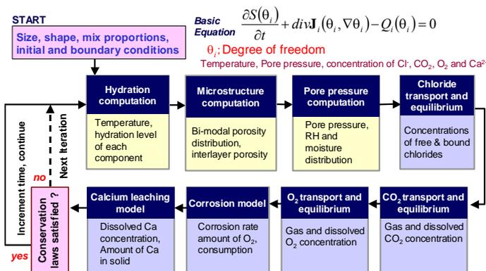
Figure 28. Sub-structure platform of Concrete Model for Durability -DuCOM-
