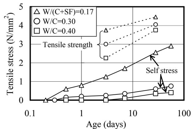
Figure 12. Restraint stress in RC beam specimens (100x100x1200mm, Steel ratio: 2.77%).
