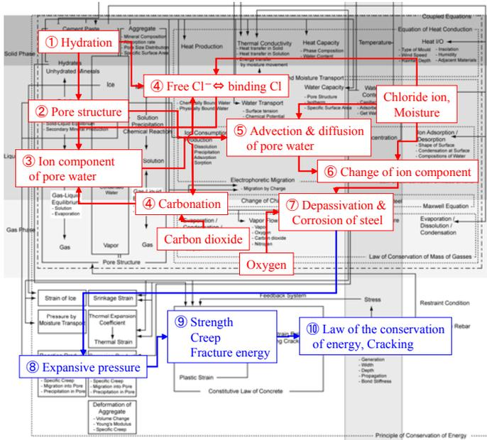
Figure 8. Durability mechanics related to crack due to corrosion of steel.
