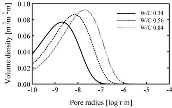
Figure 15. Assumed pore size distribution for calculation of shrinkage of specimens.
