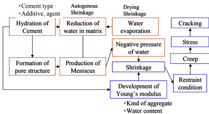
Figure 4. Process of cracking due to shrinkage.
