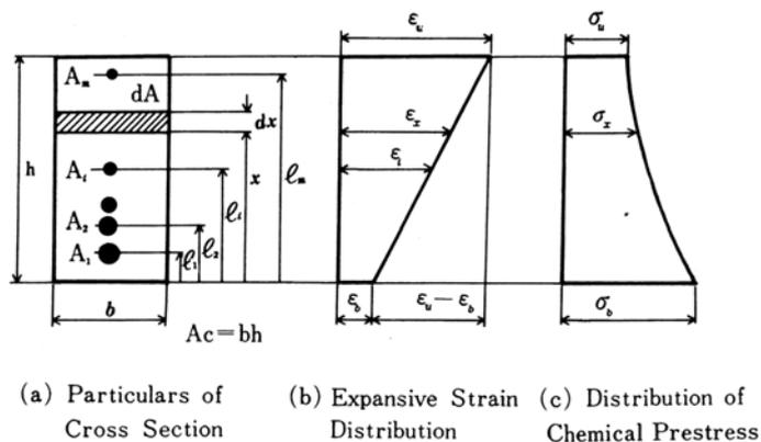
Figure 13. Estimation of distributions of expansive strain and chemical prestress.
