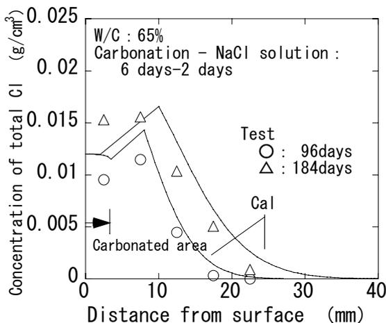
Figure 19. Prediction results of  $\text{Cl}^-$  distribution under salt damage and carbonation condition.
